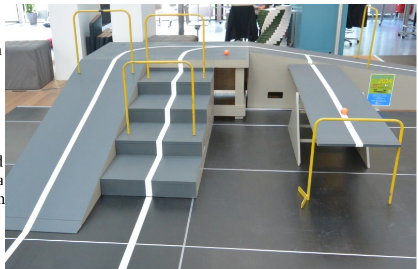
Figure 4: Ramp, plateau, staircase and seesaw. the orange golf balls on the platform and seesaw are just visible. The floor is dark with narrow aluminium edges.
