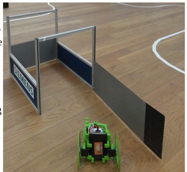
Figure 6: Tunnel with the wide door open. The doors are 1.5mm iron plates and both open outwards.
