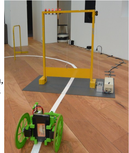
Figure 2: guillotine gate and example of a white line on the wooden floor.
