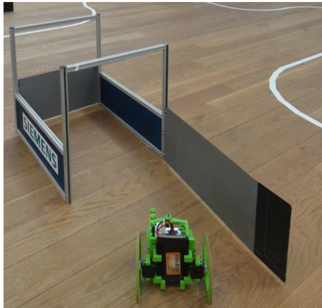
Figure 5: The tunnel with doors at each end. The wide door is open. The doors are 1.5mm iron plates and both open outwards. The ArUco codes are not shown.
