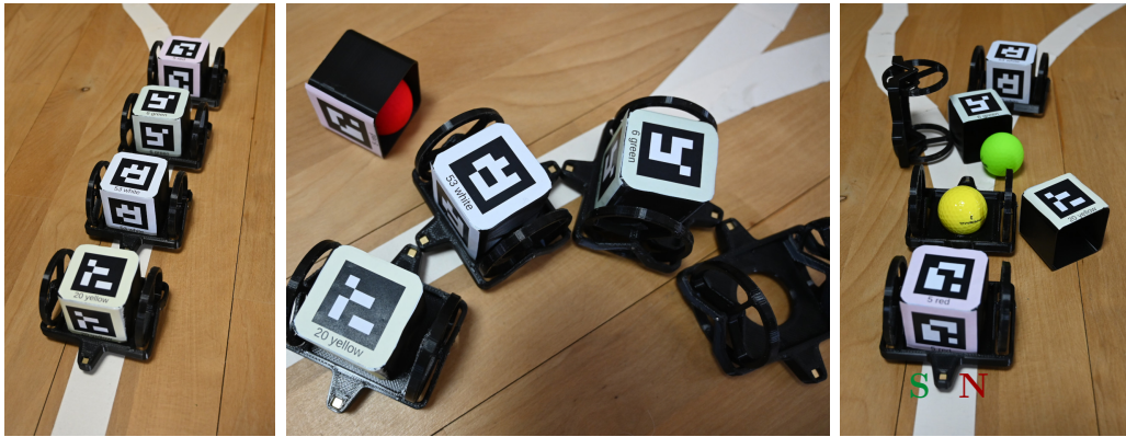
Figure 8: Package delivery trolleys. The trolleys are connected with magnets, they are marked with a delivery code. The magnets are oriented as shown in the right image.
