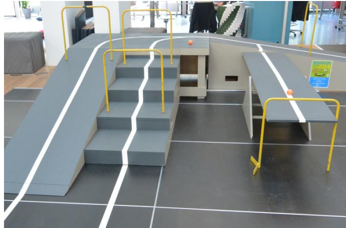
Figure 3: The figure shows the ramps, the see-saw and the stairs. The orange Golf balls and the yellow gates are visible, too. Notice also the aluminium edge of the floor plates.
